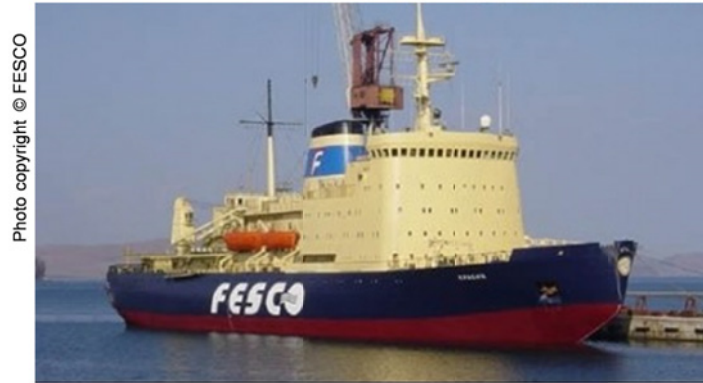
Figure 6-9: Example of a Medium-Powered Icebreaker – the Fesco Krasin
