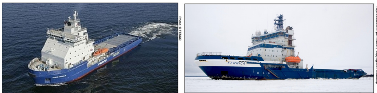
Figure 6-10: Examples of Ice-Strengthened Supply Vessels – the Fesco Sakhalin and the MSV Fennica
