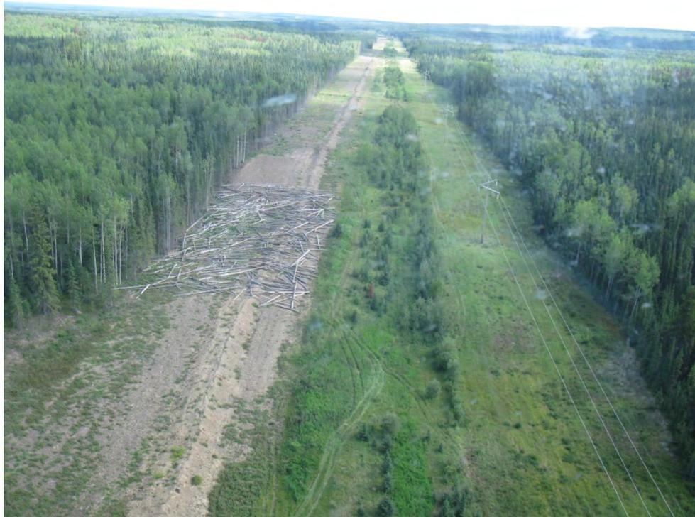
Plate 4: Example of access control implemented on a ROW with parallel developments. Note the ATV tracks that divert around the woody debris rollback. Photo source: NGTL
