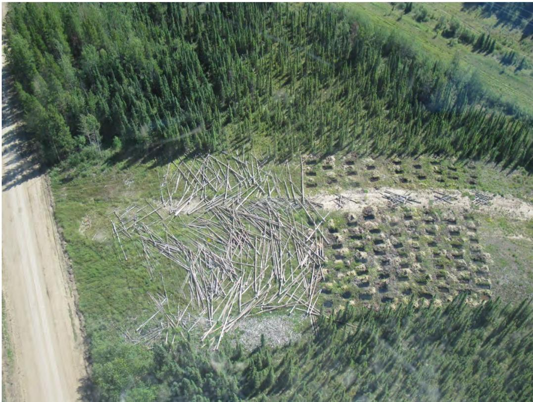
Plate 6: Aerial view of combination rollback and mounding as access control on a non-parallel portion of the ROW. Photo source: NGTL.
