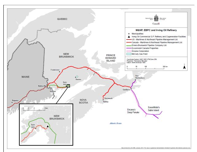
Figure 1-1: Map showing both M&NP and EBPC pipelines
