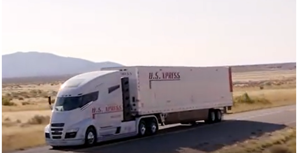
Figure 6: Prototype Nikola One hydrogen truck with 800 km to 1600 km range with 15-minute refill time. Source: Nikola Motors
