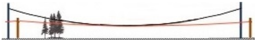
Figure 8: Reducing visual impact of high voltage transmission lines with high tension low sag conductors
